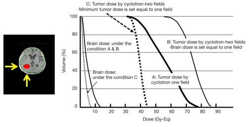
Figure 4 DVH (dose volume histogram) comparison of one field vs. two fields.
